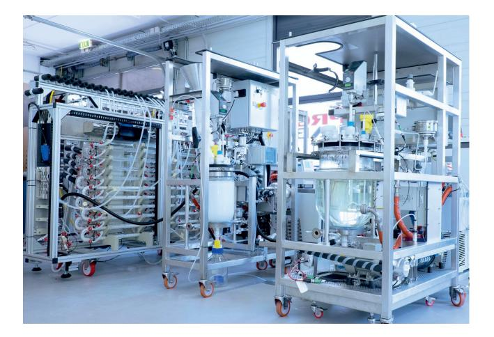
The delivered plant systems are thoroughly used at the research institutions to develop efficient crystallization processes for API's and intermediates in pharmaceutical production. The delivered continuous crystallization plants were specifically designed for research purposes. With a capacity of 1-8 L/h, the modules are fully automated and were prepared for PAT integration such as FBRM and RT microscopy allowing for model predictive control (MPC).
